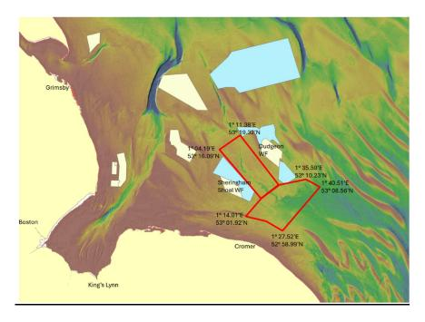
This will consist of the deployment of a vibrocorer, seabed samplers, short geological dredges and seismic surveying. During the survey, equipment will be towed behind the vessel at max 100m.
